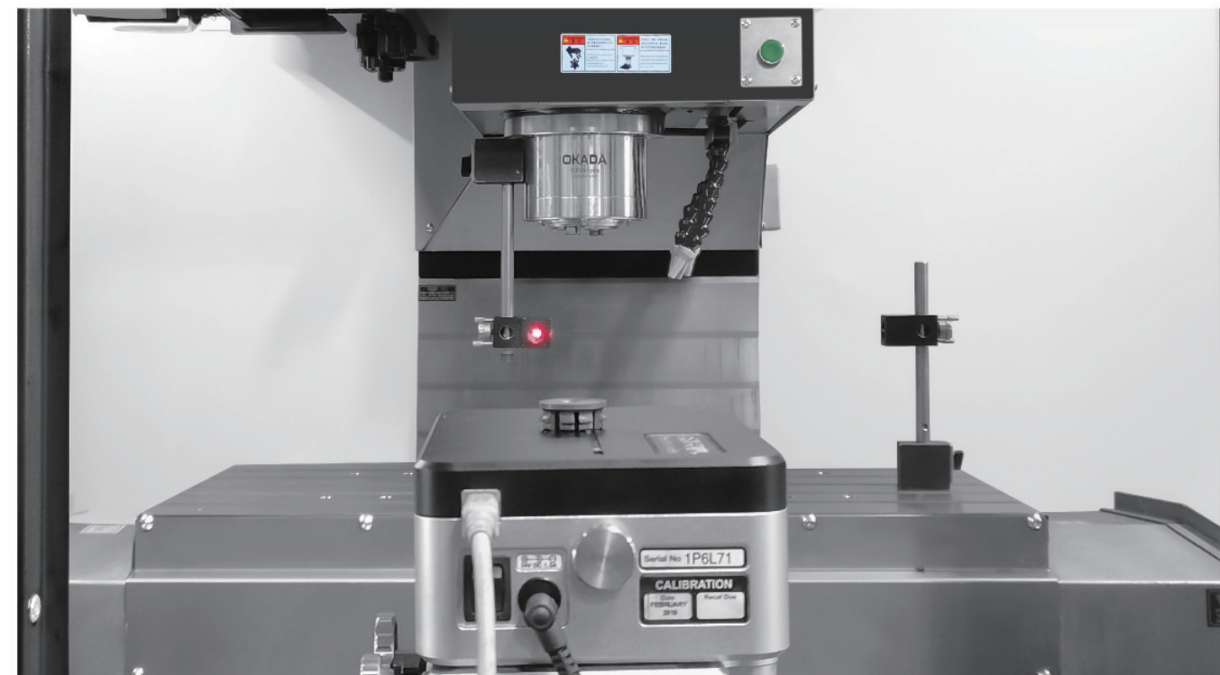
▲ 镭射检验 Laser inspection 采用英国Renishaw球杆仪做循环测试，出机前全检，确保机械精度 Using the British Renishaw club tester for cyclic testing, conduct a full inspection before leaving the machine to ensure mechanical accuracy
